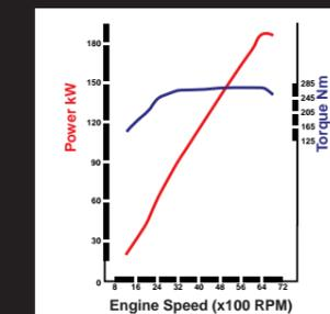
*Powerful 184kW engine in 6 speed manual*
