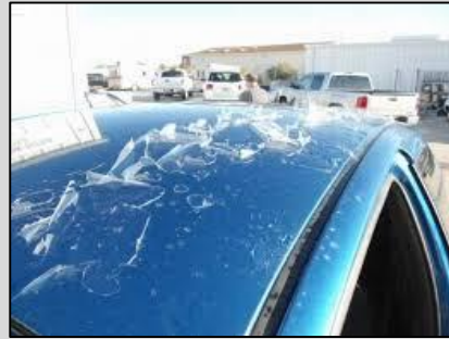
Clear Coat - Peeling
