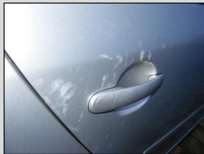
Exterior Sunscreen Damage
