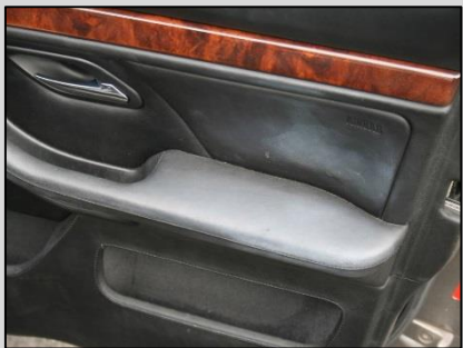
Interior Sunscreen Damage
